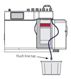
Open filter door, uncoil flush line. Direct flush line into bucket.
