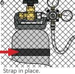
Turn on the cylinder valve Adjust outlet pressure 3.0 bar.
